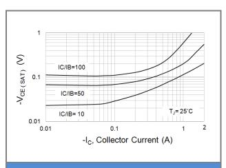
Fig.3 Typical Collector-Emitter Saturation
