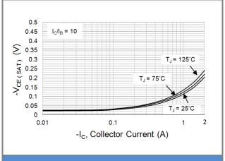
Fig.4 Typical Collector-Emitter Saturation
