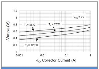
Fig.2 Typical Base-Emitter Turn-on Voltage
