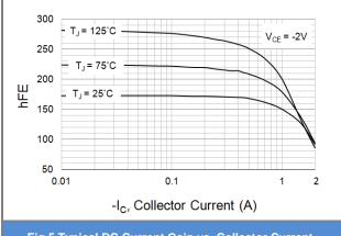
Fig.5 Typical DC Current Gain vs. Collector Current
