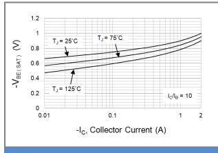
Fig.1 Typical Base-Emitter Saturation Voltage
