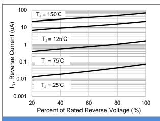
Fig.3 Typical Reverse Characteristics
