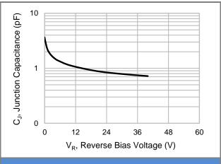
**Fig.2 Typical Junction Capacitance**
