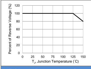
**Fig.5 Operating Temperature Derating Curve**
