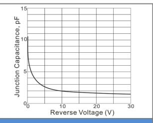
Fig.2 Typical Junction Capacitance
