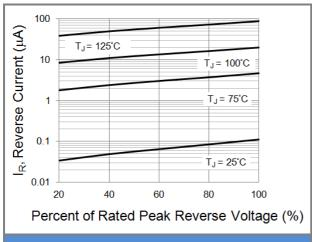
Fig.3 Typical Reverse Characteristics
