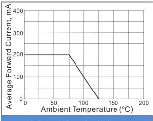
Fig.1 Forward Current Derating Curve
