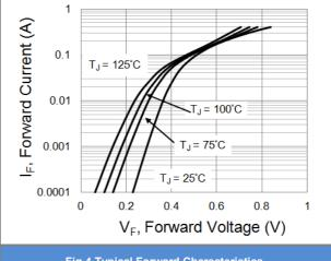
Fig.4 Typical Forward Characteristics
