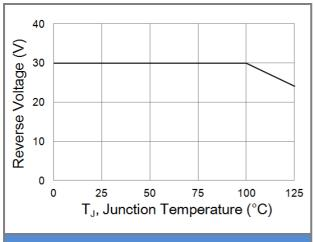
**Fig.5 Operating Temperature Derating Curve**
