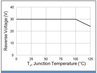
Fig.1 Operating Temperature Derating Curve
