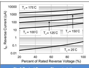
Fig.3 Typical Reverse Characteristics
