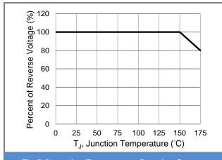
Fig.5 Operating Temperature Derating Curve
