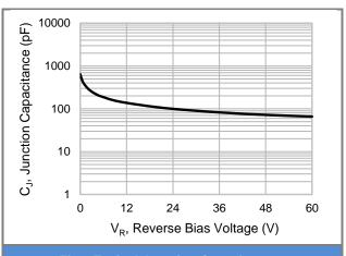
**Fig.2 Typical Junction Capacitance**
