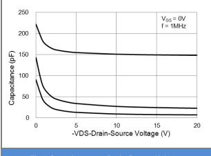
Fig.9 Capacitance vs. Drain-Source Voltage
