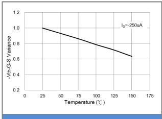
Fig.8 Threshold Voltage Variation with Temperature
