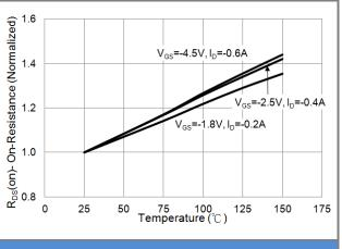
Fig.4 On-Resistance vs. Junction temperature
