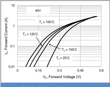
Fig.8 Typical Forward Characteristics
