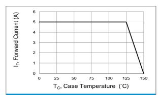
**Fig.1 Forward Current Derating Curve**
