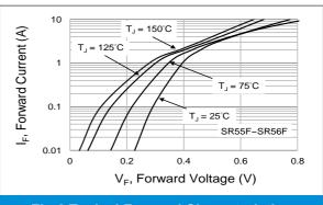
Fig.6 Typical Forward Characteristics
