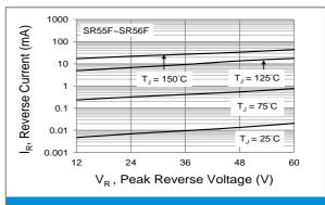
Fig.4 Typical Reverse Characteristics
