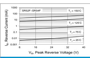
Fig.3 Typical Reverse Characteristics
