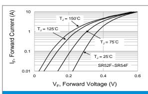
Fig.5 Typical Forward Characteristics
