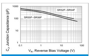
Fig.2 Typical Junction Capacitance
