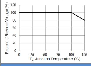
**Fig.5 Operating Temperature Derating Curve**
