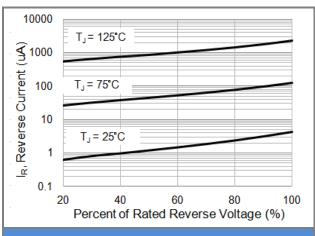
Fig.3 Typical Reverse Characteristics
