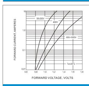
Fig.3 FORWARD CHARACTERISTICS
