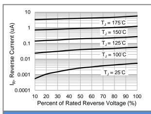
Fig.3 Typical Reverse Characteristics
