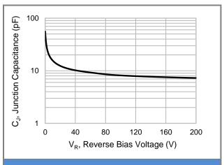
Fig.2 Typical Junction Capacitance
