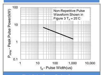
Fig.1 Pulse Power Rating Curve
