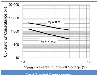
Fig.4 Typical Capacitance
