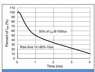
Fig.3 10/1000us Pulse Waveform
