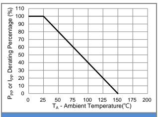
Fig.2 Derating Curve
