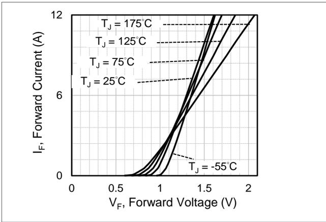
Fig.1 Forward Characteristics
