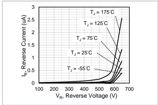
Fig.2 Reverse Characteristics
