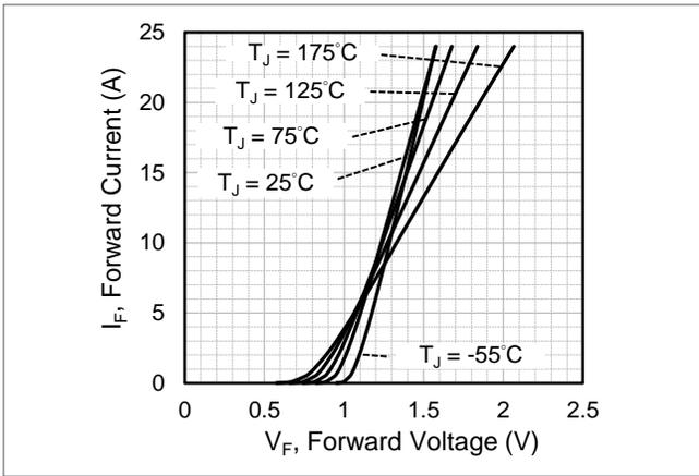
Fig.1 Forward Characteristics
