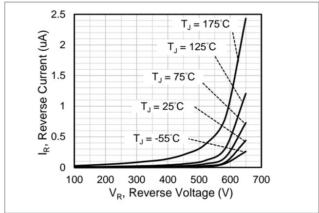
Fig.2 Reverse Characteristics
