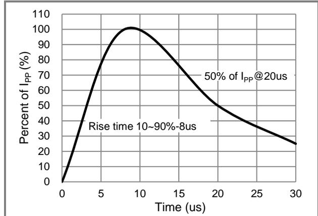
Fig.2 Pulse Waveform
