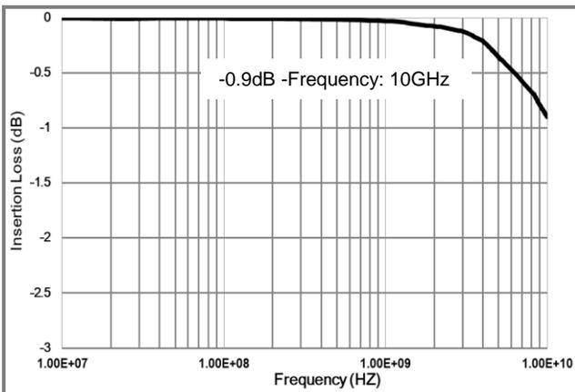
Fig.5 Insertion Loss
