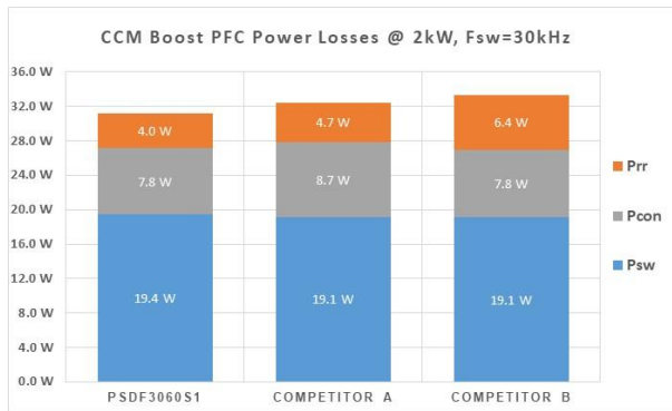
(c) Power loss @ 2kW, 110Vac, 400VDC,
