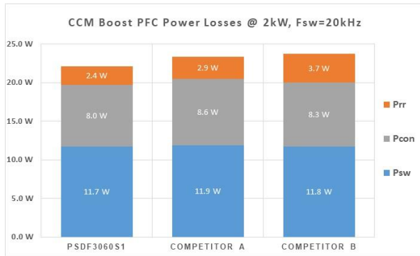
(a) Power loss @ 2kW, 110Vac, 400VDC,
